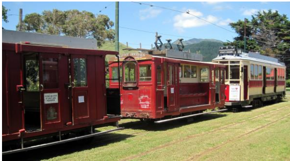
Above: Tram 151 (4 foot gauge) assisted in hauling out the cable car and trailer (each 3ft 6" gauge) on our multi-gauge track.
