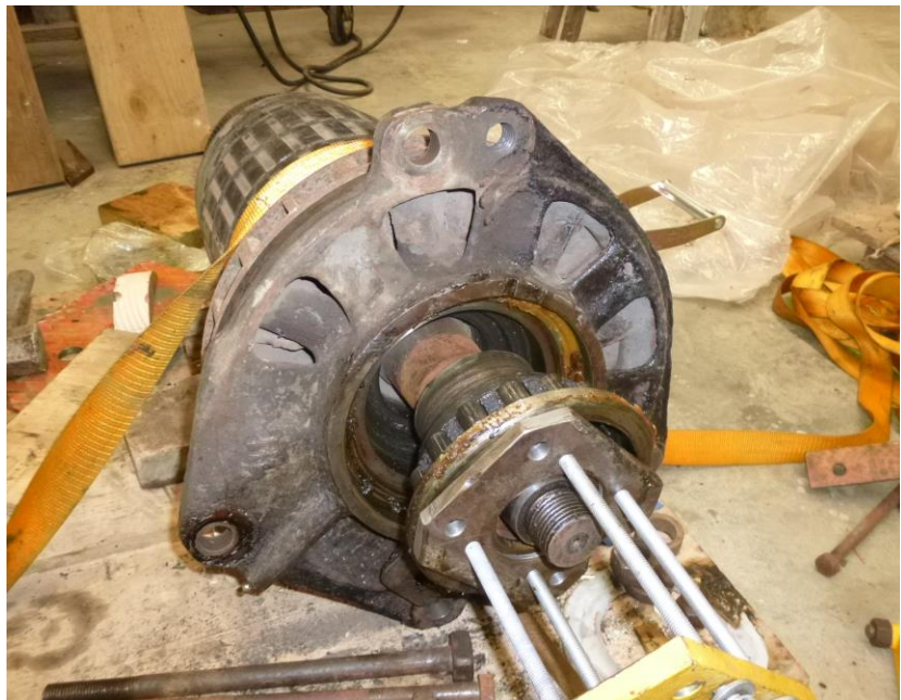
The bearing on the pinion end of the motor was most resistant to removal – shown here finally removed on 4 th January. Photo: Colin Dash
