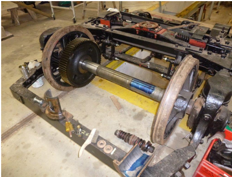
The "A" end truck for tram 260 (ex tram 235) with motor removed and showing the driving axle
