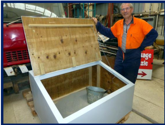
Above: The new tram sand storage bin. This has now been moved to the front of barn road 3, in front of the mock-up tram cab, and has been brought into use.
