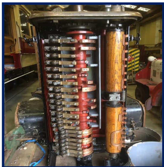
Above: the first of the BTH B510 controllers - restored for tram 17 by Trevor Weaver.
