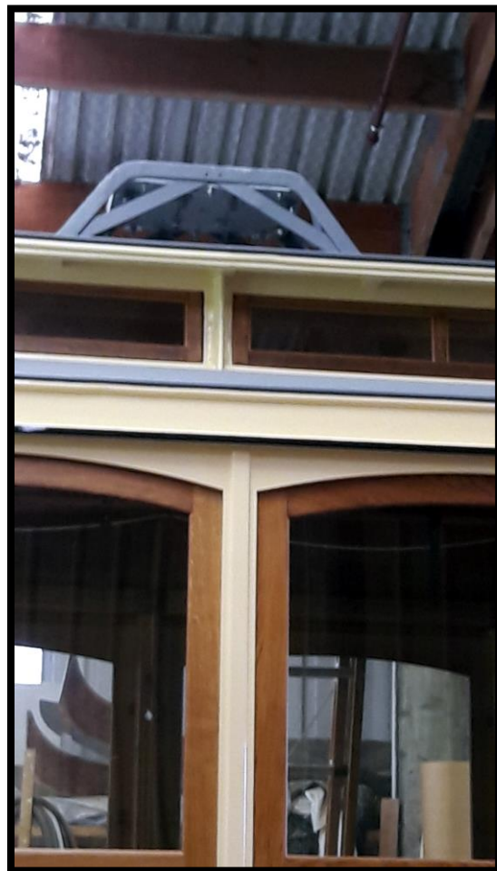
Above: 7 th April, and the trolley tower is mounted on the tram.
