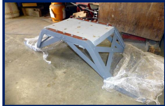
Above: The trolley tower height has been reduced by removing the raised sides.
